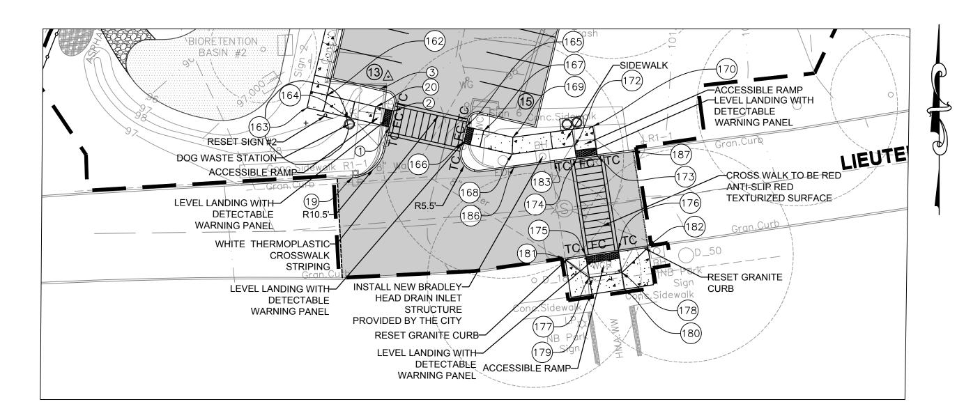
ADDENDUM 2 - FULLER PKWY SIDEWALK, CURBS AND RAMPS SITE LAYOUT & MATERIALS PLAN SCALE: 1"= 20'-0"
