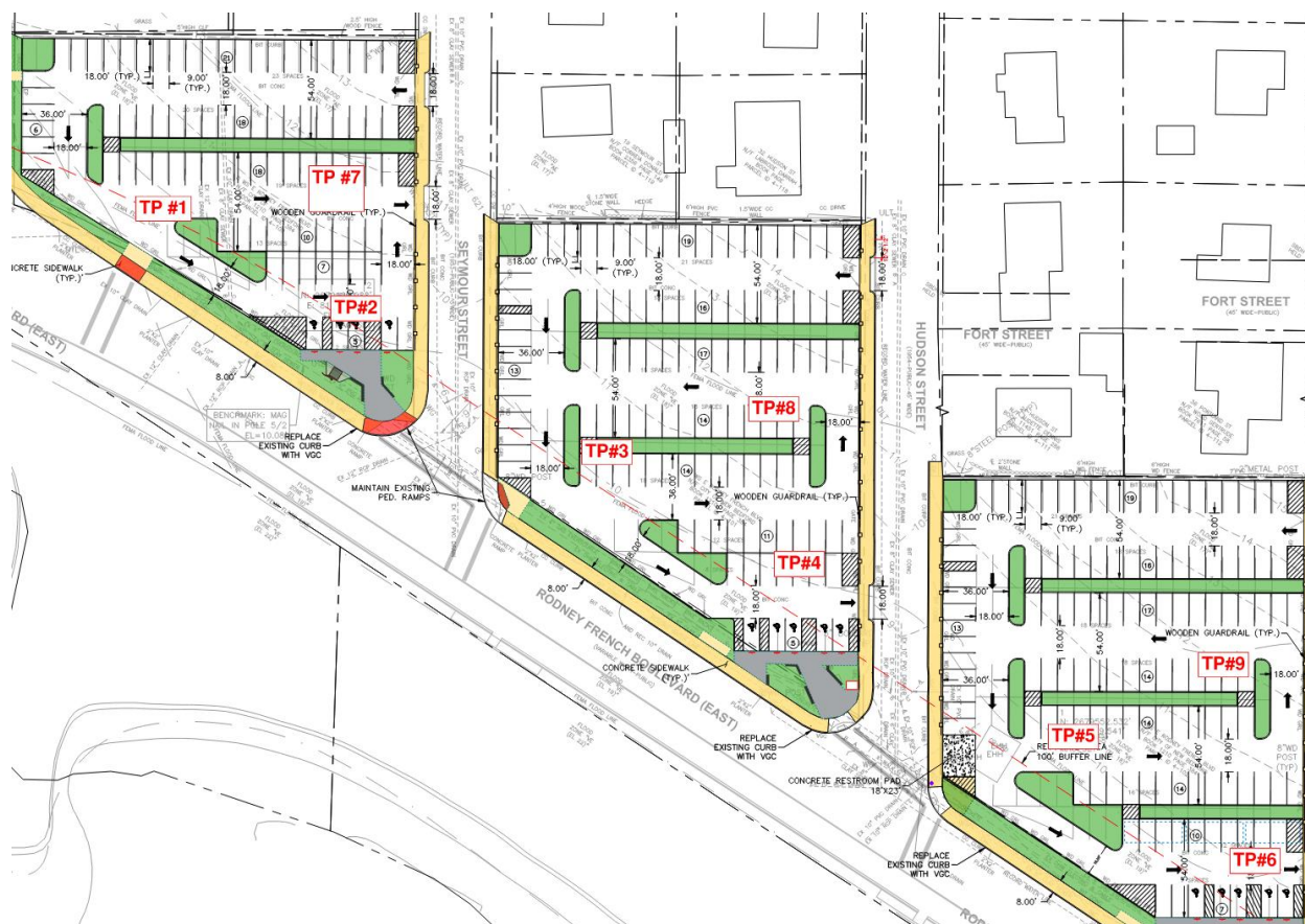
Figure 3: Test Pit Locations
