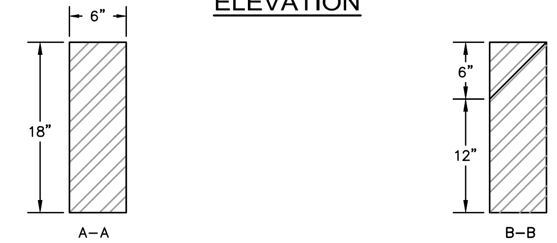
GRANITE TRANSITION CURB DETAIL VERTICAL TO SLOPE NOT TO SCALE A DERIVATIVE OF MDOT 106.4.0
