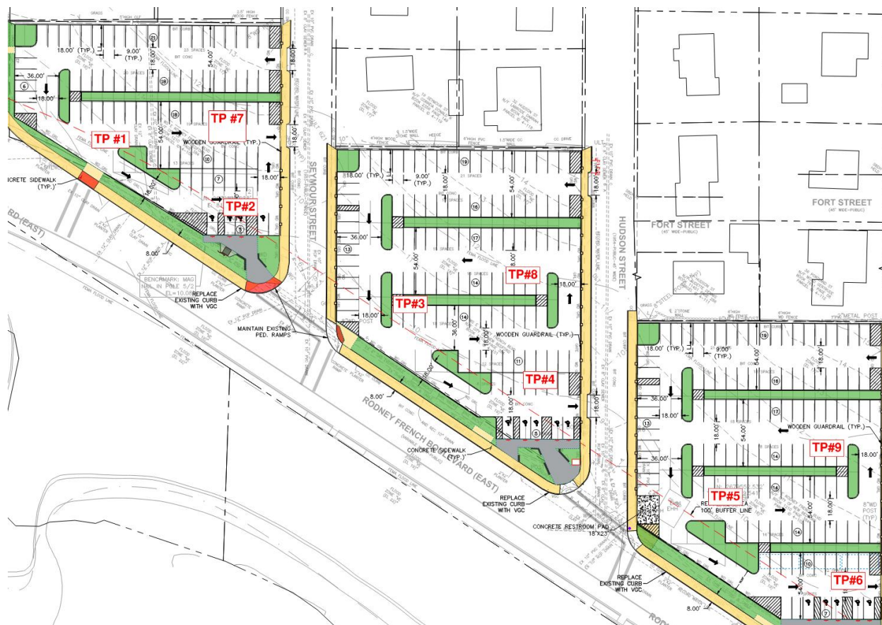
Figure 3: Test Pit Locations
