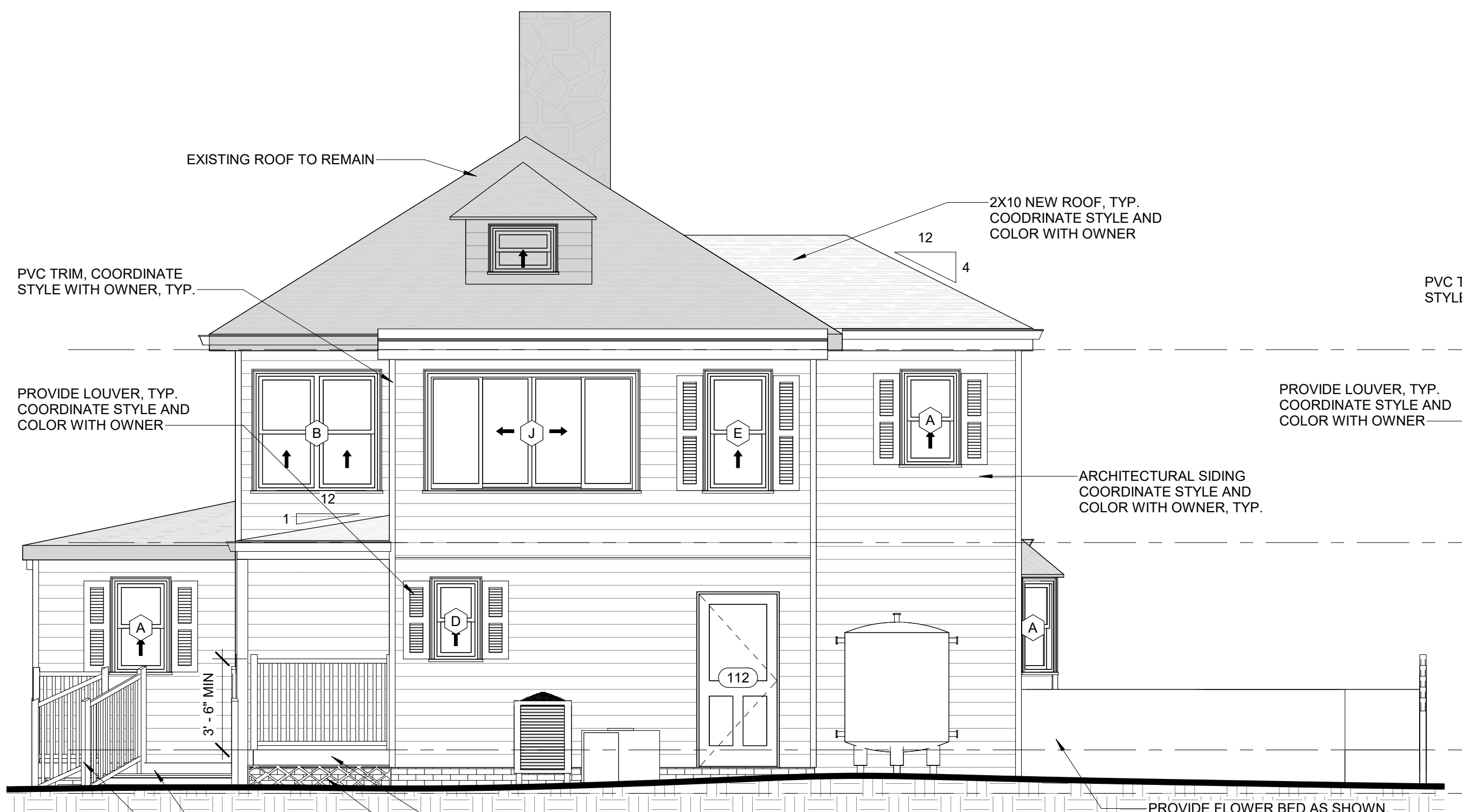
3 PROPOSED WEST ELEVATION 1/4" = 1'-0"
