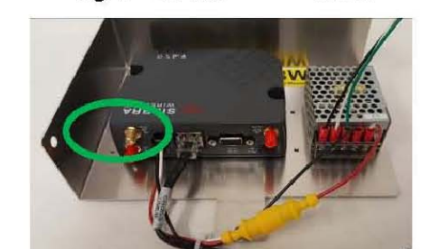
Fig. 3 – 4G Modem Connection
