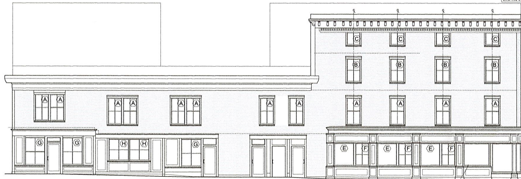
WEST ELEVATION - PROPOSED SCALE: 1/8" = 1'-0"
