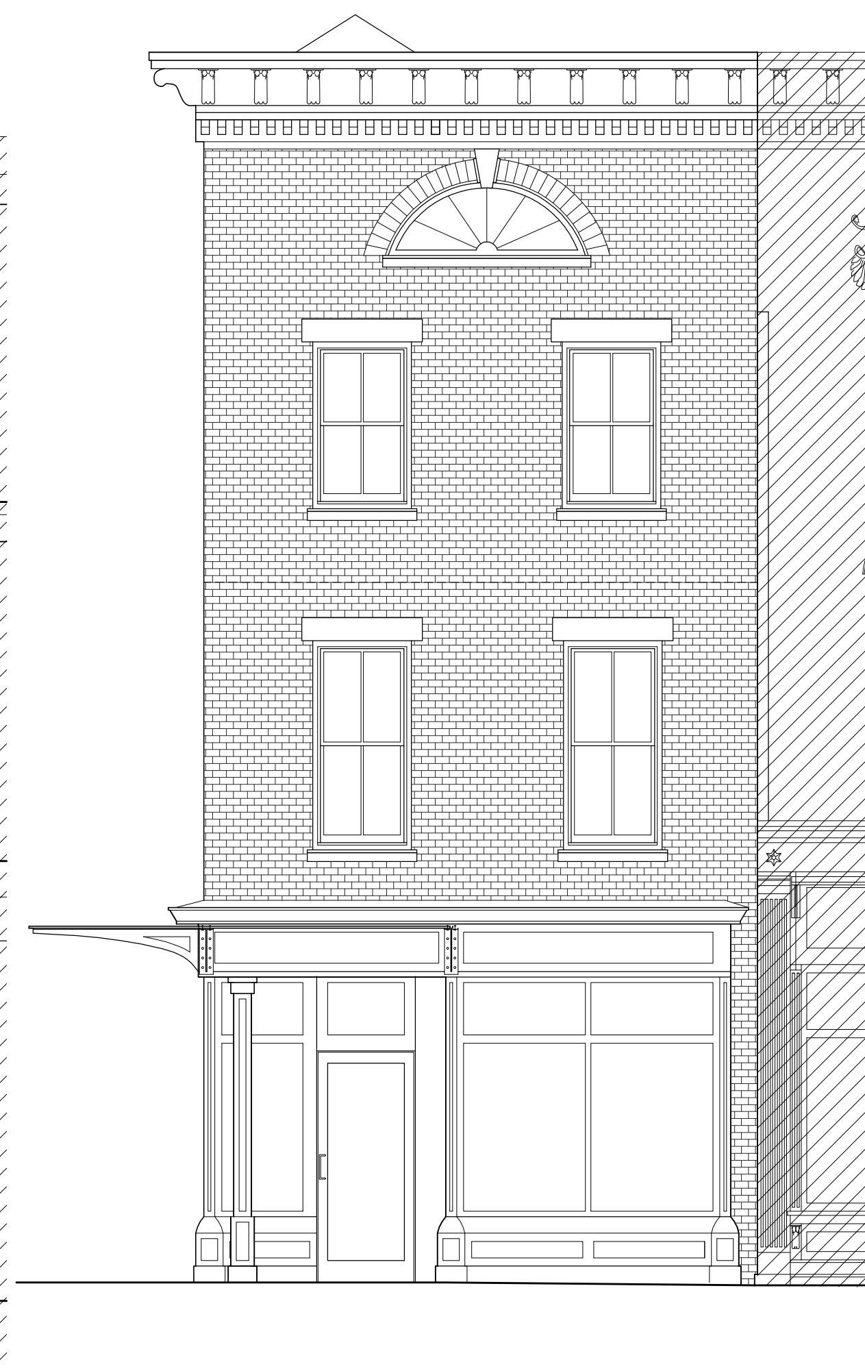
PROPOSED ELEVATION - UNION STREET - SOUTH SCALE: 1/4" = 1'-0"
