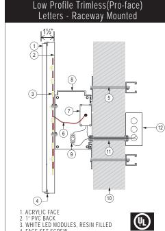
3. WHITE LED MODULES, RESIN FILLED 4. FACE SET SCREW
