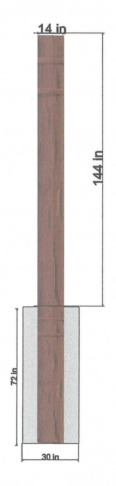
Utility poles are buried according to a particular formula 10 percent of the pole's height plus two feet equals the appropriate depth of burial. 18 feet - 10% 18" + 24" = 42"
