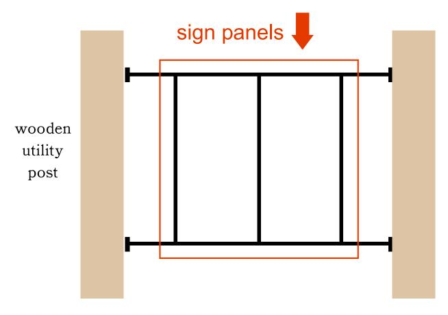
steel frame system 1 x 1 two single sided sign panels affixed to frame system with galvanized nuts and bolts
